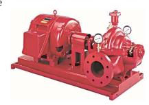
pump is covered by a "split" casing, which can be opened for pump maintenance. The impeller is connected to the drive by a horizontal shaft. This type of pump is very reliable and available in a wide range of flow and pressure ranges. Unfortunately, this style of pump, typically, requires the largest floor space also.
