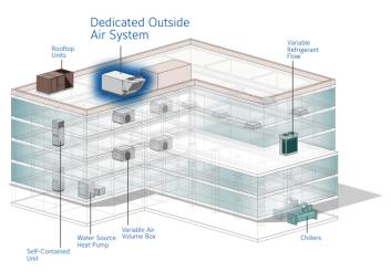
beneficial to pretreat the ventilation air at a central location. A centrally located DOAS is often used to heat and cool ventilation air to "room neutral" conditions, i.e. approximately the same temperature (and often humidity) as the room air, so the terminal equipment does not need to condition it<sup>2</sup>.
